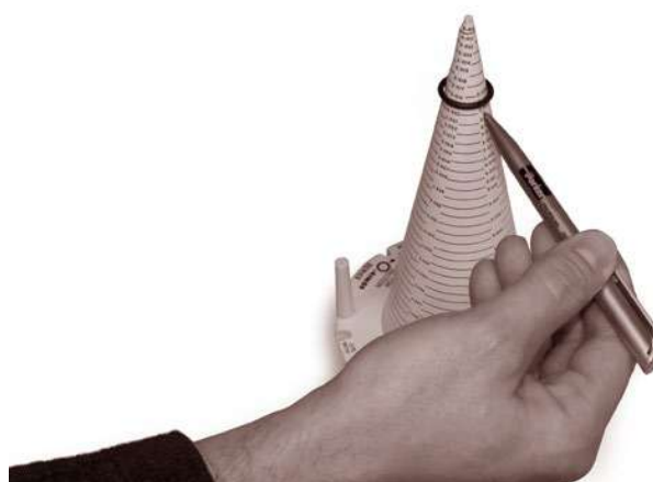
Fig. 5.4 Determination of the 2-xxx size number with the measuring cone
