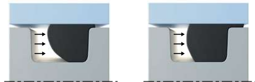
Fig. 10.3 At higher pressure a larger O-ring volume is pushed into the gap. A back-up ring prevents gap extrusion.
