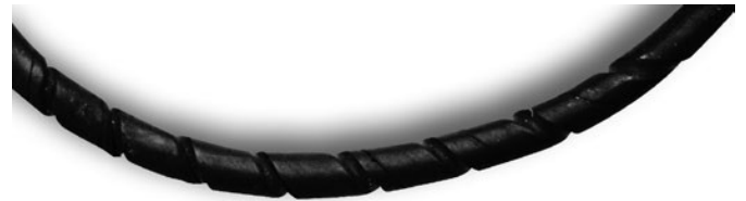
Fig. 10.9 Twisted O-Ring with spiral markings
