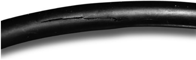
Fig. 10.11 O-Ring damaged by explosive decompression
