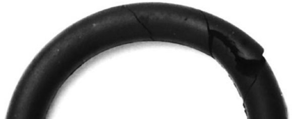
Fig. 10.10 Twisted O-Ring with cuts in surface
