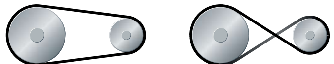
Fig. 2.18 Open design (left), crossed design (right)
