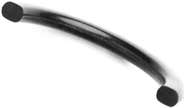
Fig. 10.8 Damage pattern caused by high compression set
